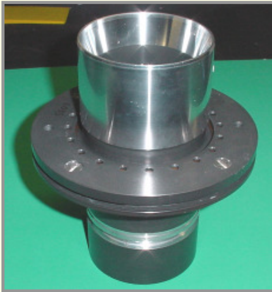
Refurbished & redesigned Piston for DL(V)F-K with H.P. Injection Valve
