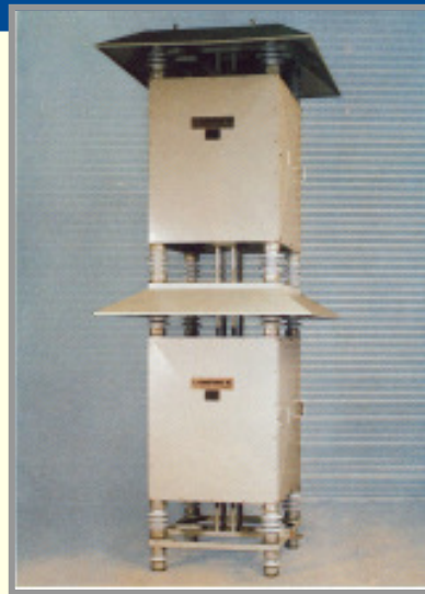
Filter Resistor for Pacific HVDC Inter-Tie, USA; Single-Phase 57 \Omega , 30 kW BIL 450 kV across Resistor, 500 kW Inductivity < 20 \mu H Seismic Withstand 0.5 g Resistors of this type are in operation up to 800 kW, LIWL up to 650 kV.
